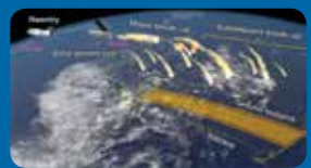
Structural breakup upon re-entry into dense atmosphere, most of the materials ablate except a few components (gas bottles, tanks, nozzles)
