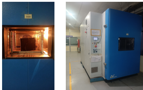
Fig-2: Pictorial view of Vertical type thermal shock chamber used for solar coupon testing
