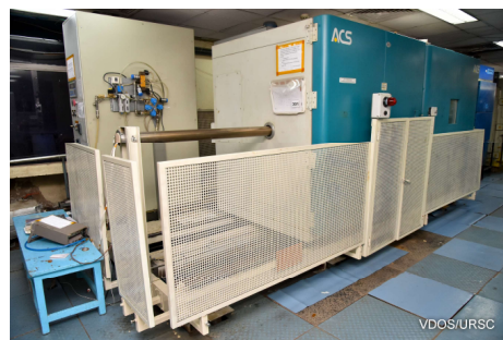
Fig-3: Pictorial view of Horizontal type thermal shock chamber used for solar coupon testing
