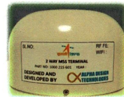
MSS Xponder for Coastal Monitoring, enables periodic position reporting, two-way messaging, boundary crossing alerts and emergency broadcast reception system for maritime domain
