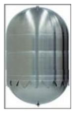
The volumes of PS4 propellant tank (for 4th stage PSLV) varies from 1,600 litres to 3,000 litres approximately. The diameter is 1,380 mm. This is a bi-compartmental propellant tank with Propellant Acquisition System (PAS). In this case also the thin walled, machined semi elliptical end-dome and cylindrical-shells are electron beam welded to realise the propellant tanks.
