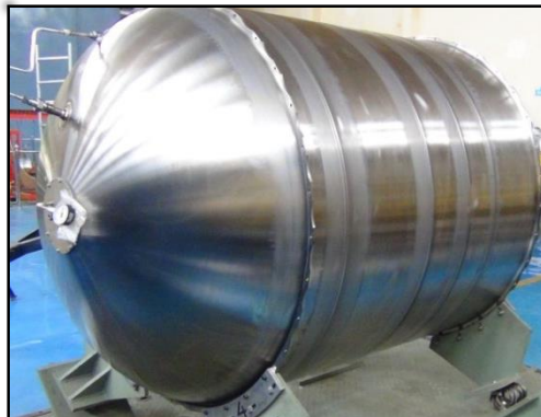
PS4 PROPELLANT TANK (Dia.1380mm)
