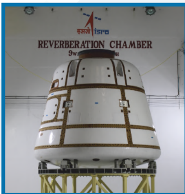
Crew Module Acoustic Test at ISITE, URSC
