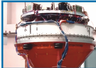
Equipment Bay vibration test
