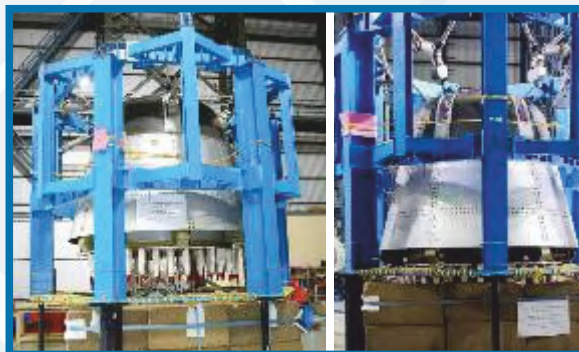
Crew Escape System separation test
