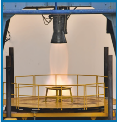
AR 6 VIKAS Engine hot tests
