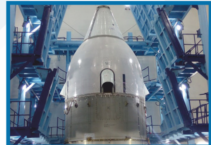
CES Ground Resonance Test
