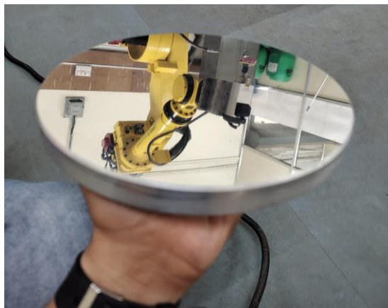
Robot-Assisted Polishing Setup and the Polished mirror surface manufactured
