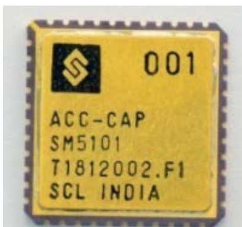
micro-g class MEMS Accelerometer with close loop Readout Integrated Circuit (ROIC)
