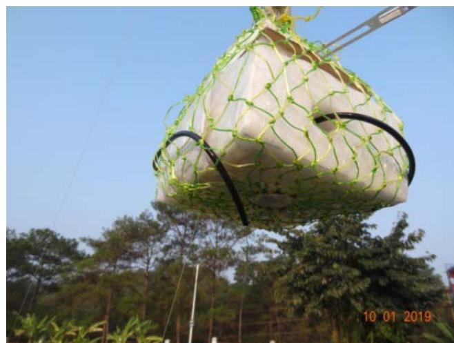
Fig. 1: Hydrogen gas filled tethered balloon (left) and instrumented payload connected with the tethered balloon (right)
