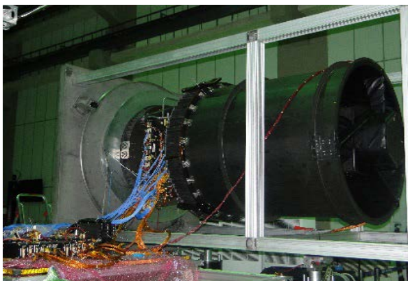
Fig.3: Carto-3 EOM integrated with Payload Electronics & FPA
