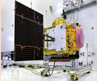
**IRNSS-1D undergoing solar panel** deployment test
