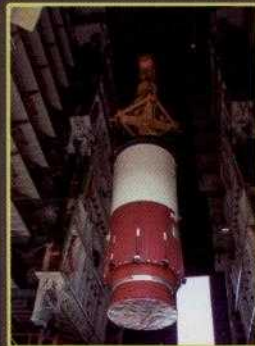
Core Base Shroud + Nozzle end segment stacking at VAB
