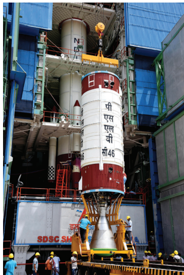
Hoisting of PSLV-C46 Liquid second stage
