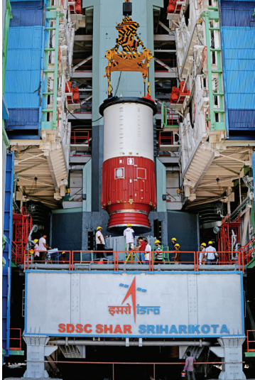
Hoisting of the nozzle end segment of PSLV-C46 first stage over the launch pedestal
