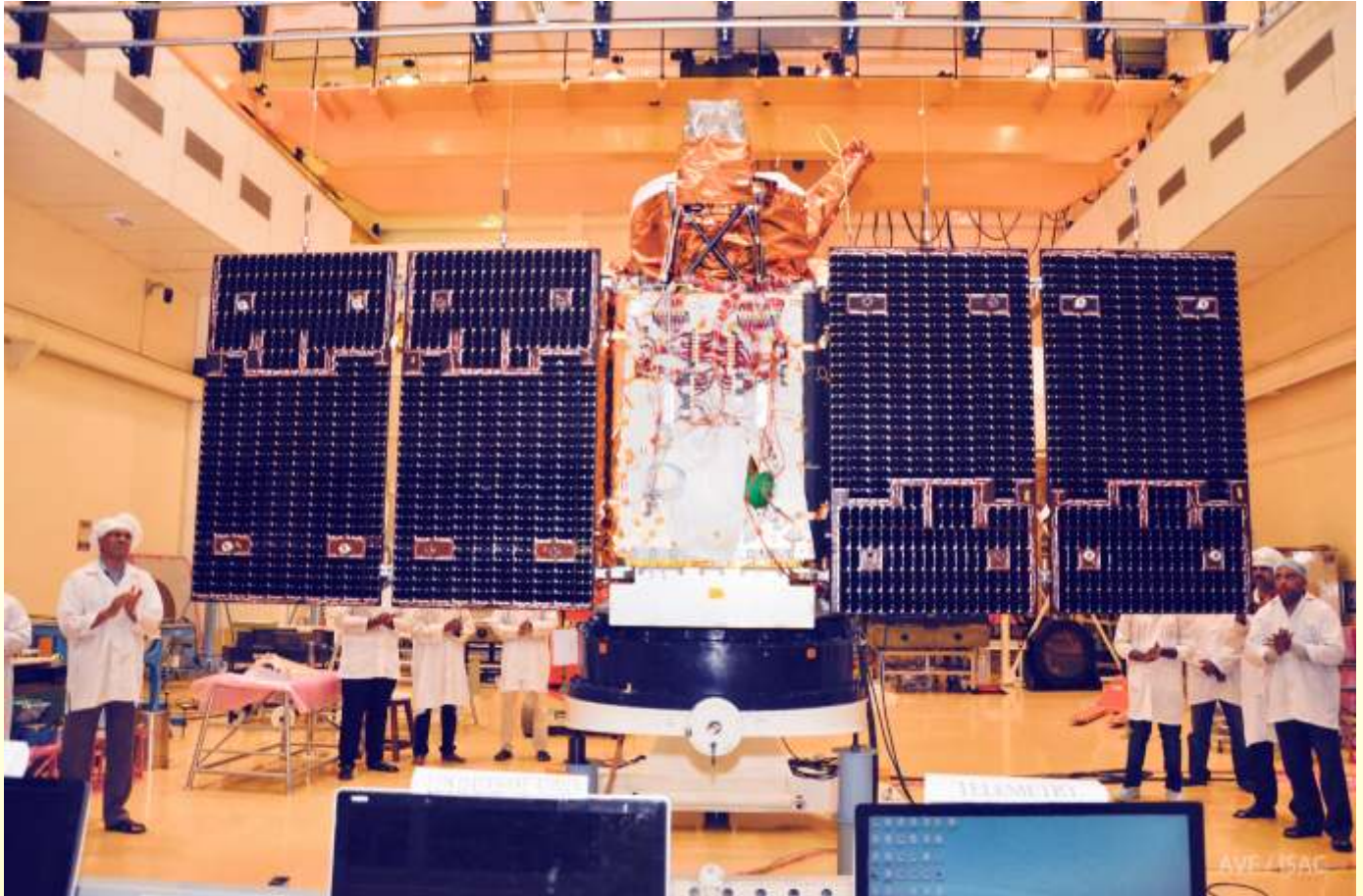
Cartosat-2 series satellite undergoing panel deployment test
