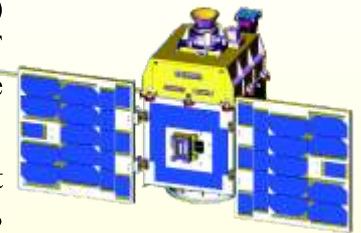
INS-1A Deployed Configuration with SBR/Single Event Upset Monitor (SEUM) payload
