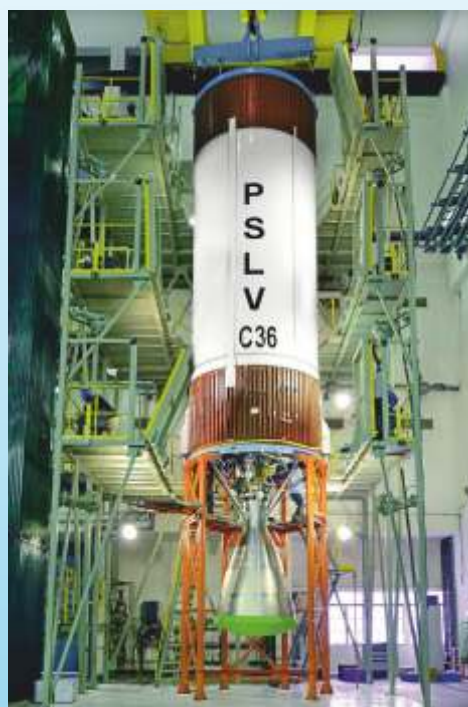
PSLV-C36 second stage (liquid) at Stage Processing Facility
