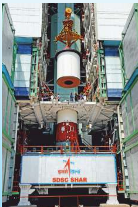
Hoisting of a segment of PSLV-C36 core stage during vehicle integration
