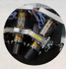
• Terrain Mapping Camera - 2: Will generate a Digital Elevation Model (DEM) of the entire Moon
