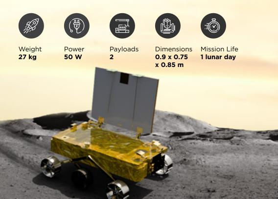
Chandrayaan 2's rover is a 6-wheeled robotic vehicle named Pragyan, which translates to 'wisdom' in Sanskrit. It can travel up to 500 m (0.5 km) at a speed of 1 centimetre per second, and leverages solar energy for its functioning. It can communicate with the lander.
