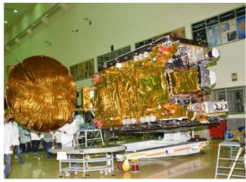
GSAT-31 Antenna Reflector Deployment test
