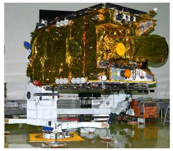
Centre of Gravity Test of GSAT-31
