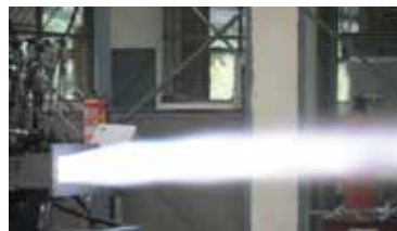
Supersonic combustion flame with GH2 & Isrosene
