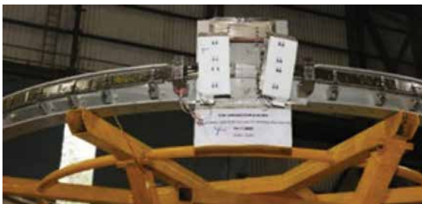
Functional test of Crew Module Fairing Separation System
