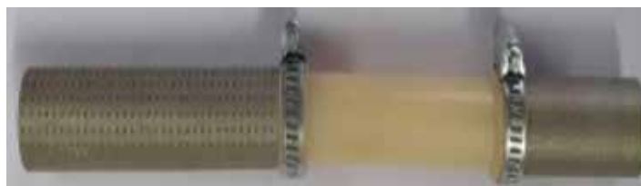
Flexible Heat Pipe developed by STIC at NIT Tiruchirappalli under mentorship of SAC, Ahmedabad
