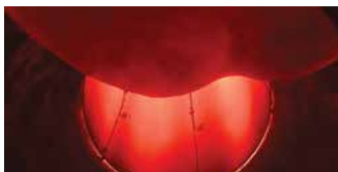
Qualification hot test of PS4 Engine with Carbon-Carbon Nozzle Divergent
