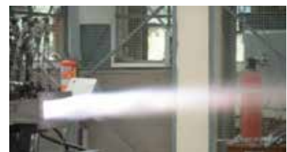
Supersonic combustion flame with Isrosene alone
