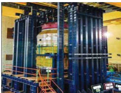
Integrated Structural Qualification Tests of Orbital Module Adaptor (OMA) & Service Module Fairing (SMF)
