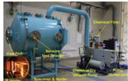
Ablative Testing vacuum chamber
