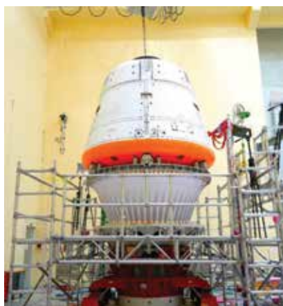
Vibration test of TV-D2 Crew Module
