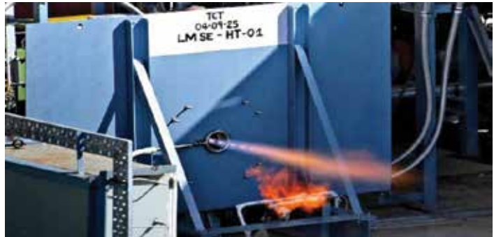
Hot Test of LOX-methane Single Element Thrust Chamber with Injector Head
