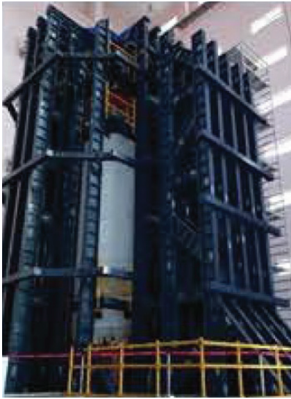
Structural Qualification test of LH2 tank with Closed ITSc and FSA
