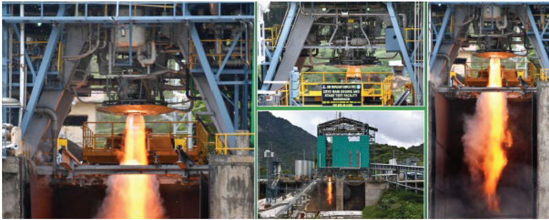
CE22 Engine Hot test
