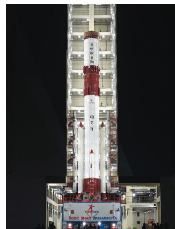
First launch vehicle integration at PIF
