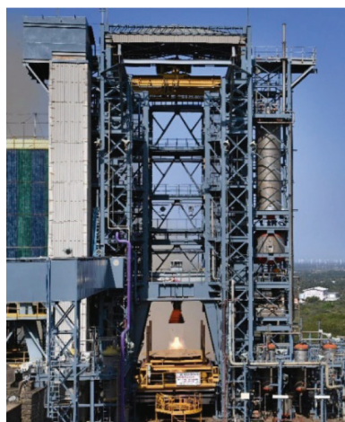
L110 Vikas engine hot test
