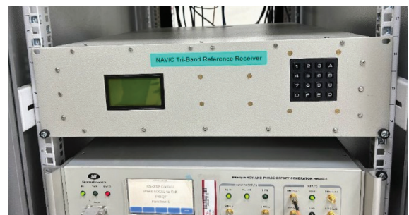
Indigenous tri-band reference receiver in NavIC ground segment
