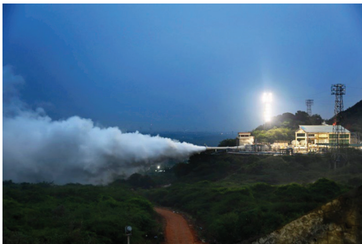
Flight Acceptance test of E12 Engine for G1 mission in High Altitude test facility
