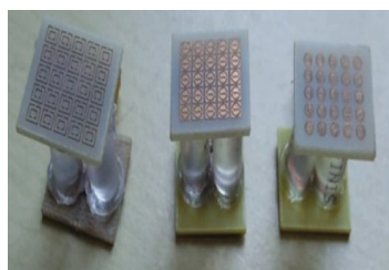
Metamaterial based Antenna developed by STIC NIT Agartala in mentorship of NESAC
