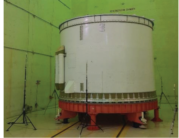
Acoustic Test on the SITS Structure
