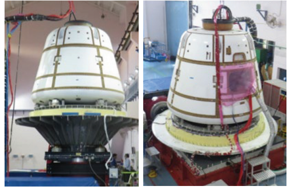
Completion of TV-D1 CM Vibration Tests at VTF, SHAR
