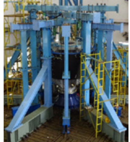
Structural Test of Crew Module
