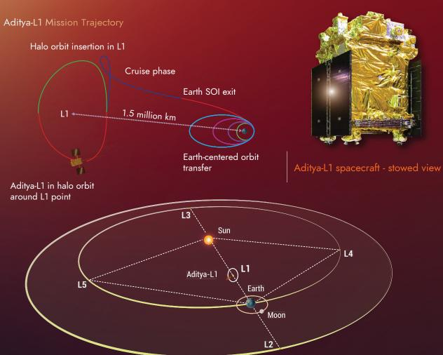
Illustration of all five Lagrange points of Sun-Earth system. The spacecraft will be placed around Largrange point 1.
