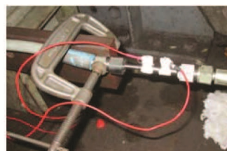
Transition Tube under Proof pressure test
