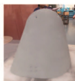
SiC coated C/C nosecap
