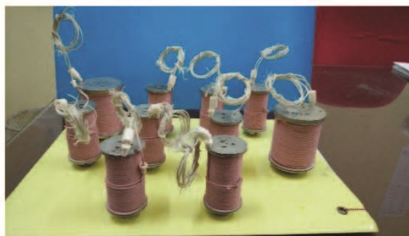
SILPOT 5052 coated bobbins for stationary plasma thruster
