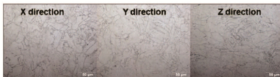
Microstructural features of 3D printed IN-718 across different printing directions
