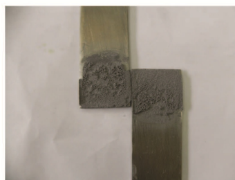
SS321 metal coupons after LSS testing
