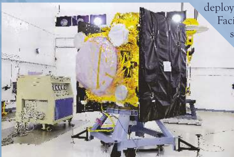
IRNSS-1E propellant filling operation in progress
